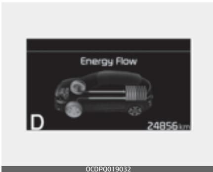
Hybrid battery is being charged by regenerative braking.
