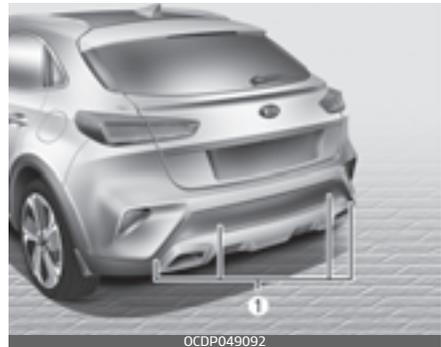
Forward/Reverse Parking Distance Warning system assists the driver during movement of the vehicle by chiming if any object is sensed within the distance of 100 cm (40 in) in front and 120 cm (48 in) behind the vehicle.
