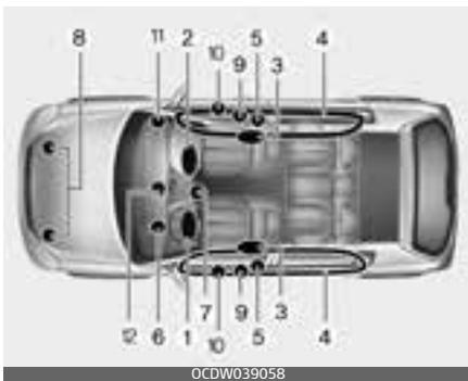
The SRS consists of the following components:
