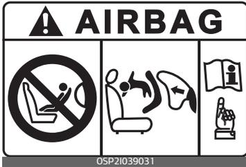
Never place a rear-facing child restraint in the front passenger's seat. If the air bag deploys, it would impact the rear-facing child restraint, causing serious or fatal injury.
