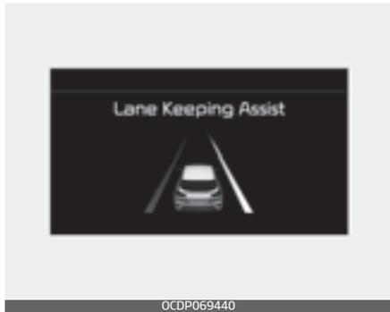
If the speed of the vehicle is over 60 km/h (37 mph) and the system detects lane markers, the color changes from gray to white.
