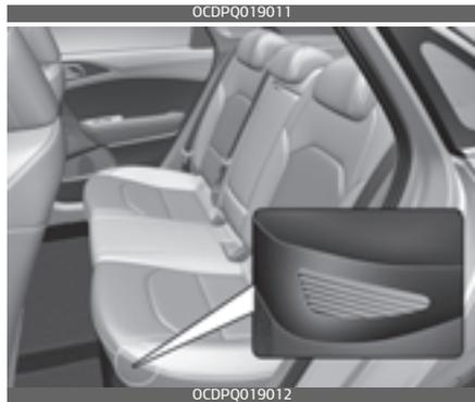
Do not put objects on the left side of rear seats. This could block the battery cooling duct causing battery degradation.
