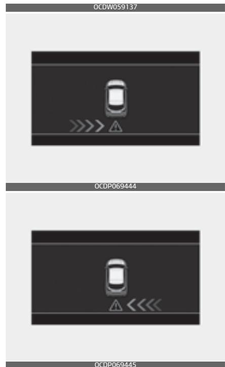
If the vehicle detected by the sensors approaches from the rear left/
