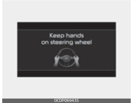
If you keep your hands off the wheel while driving with LFA system assisting the steering, the hands-off warning will be triggered.
