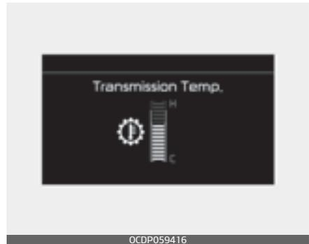
This mode displays the transmission temperature.
